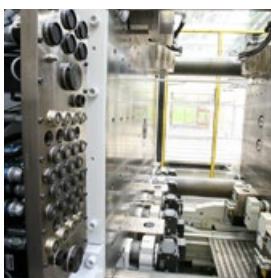
The integrated ENGEL famox (fast mould exchange) mould changing system reduces setup times, while improving machine flexibility and increasing capacity utilisation.
