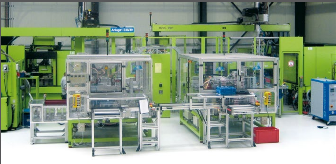
At Schneegans, two coupled injection moulding machines rely on two-component technology to produce tum.
