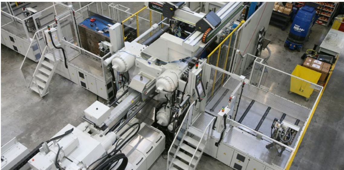
The fully automatic ENGEL famox (fast mould exchange) mould setup system ensures optimised setup times for medium batch sizes.
