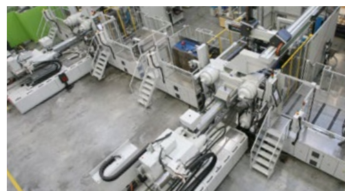
The integrated ENGEL famox (fast mould exchange) mould changing system reduces setup times, while improving machine flexibility and increasing capacity utilisation.
