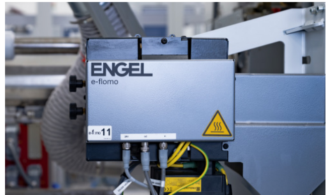
Constant temperature control for short cycle times with e-flomo.
