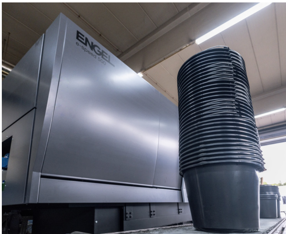
JOPA buckets made with 96% post-consumer recycled material.
