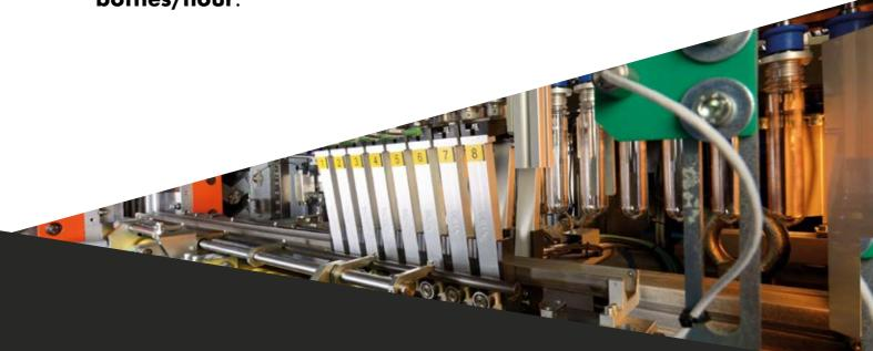
Important new features include a smart clamping unit with "dynamic stroke". Servo drives make it possible for the user to choose from three different strokes, so they can optimize output. SIPA has also further simplified the **mould changeover** procedures and has optimised the **blowing blocks** to achieve a 30% decrease in dead air volume and consequently a reduction in total air consumption.
