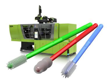
ENGEL and Hack Formenbau jointly developed and optimised the process for high-volume test swab production. The mould solution, injection moulding machine and automation are precisely tuned for maximum efficiency and quality.
