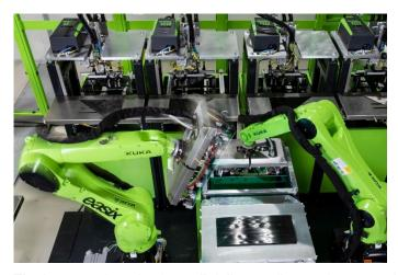
The integrated production cell delivers tailor-made composite blanks in one-minute intervals.
