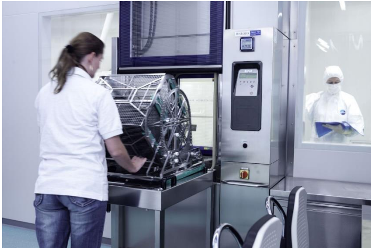
The needles for the ZipFix fasteners are fed into the clean room via an ultrapure water cleaning system. (Picture: Samaplast)
