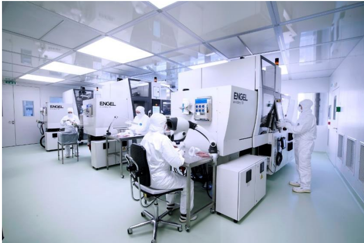
The first tie-bar-less machine was delivered to Samaplast in 1990. In the meantime, this type of machine has become established at Samaplast – even in clean rooms. (Picture: Samaplast)
