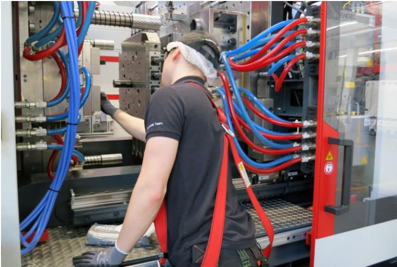
The moulds are cleaned every day. Tie-bar-less technology makes this manual work far more convenient and faster.
