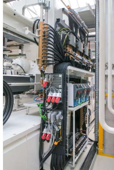
Compact integration: the production cells are equipped with e-flooms and temperature control units located on the sides and to the rear of the machine.
