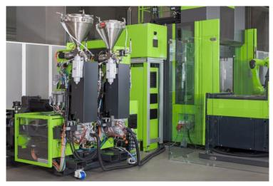
ENGEL's solution for in-situ polymerisation for the production of fibre-reinforced thermoplastic components is characterised by particularly compact system technology.
