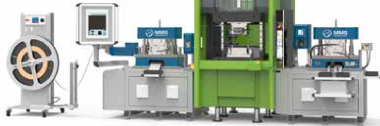
Fig. 1. The raw material for manufacturing thermal switch housings is fed directly from the reel and pre-punched, including thread tapping, in-line (© Engel/MMS)
