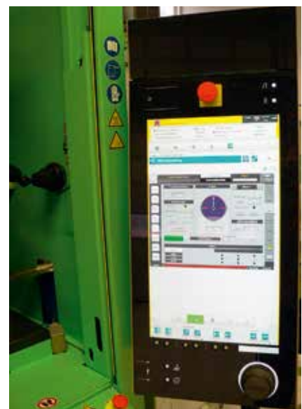
Fig. 2. Regardless of the number of modules, the entire process can be visualized and controlled via the CC300 control unit on the insert machine (© Engel)
