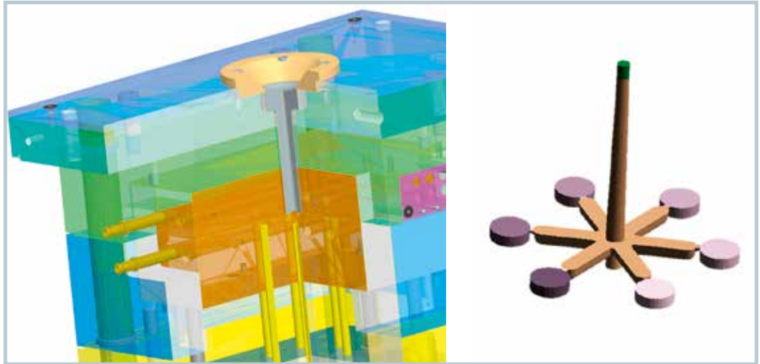
Fig. 3. Cross-section through the injection mold for pharmaceutical production (left). The tablets are connected via a star-shaped runner system with sprue gate (right)
