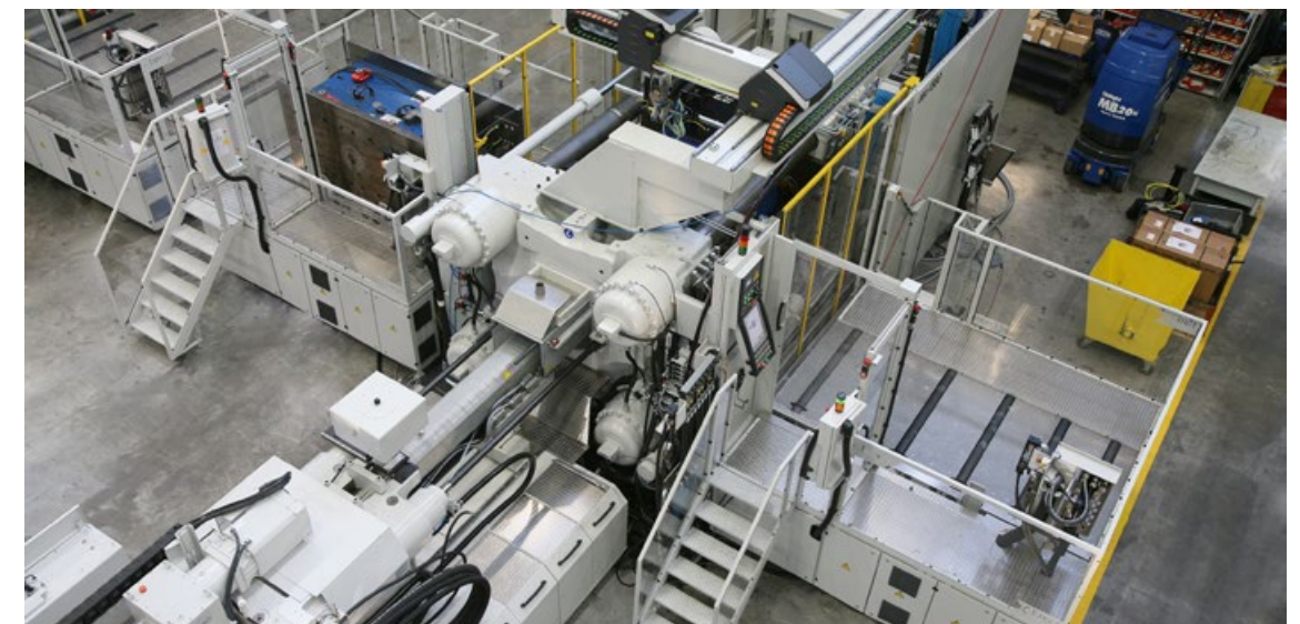
The fully automatic ENGEL famox (fast mould exchange) mould setup system ensures optimised setup times for medium batch sizes.
