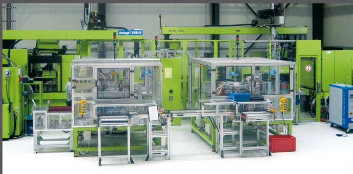
At SchneeGans, two coupled injection moulding machines rely on two-component technology to produce turn.
