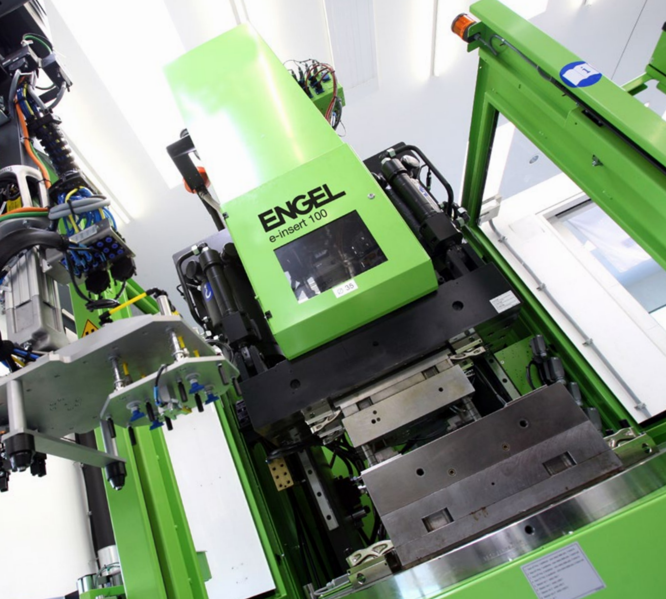
Efficiency for inserts: the ENGEL e-insert electric vertical machine combined with the powerful ENGEL viper robot.
