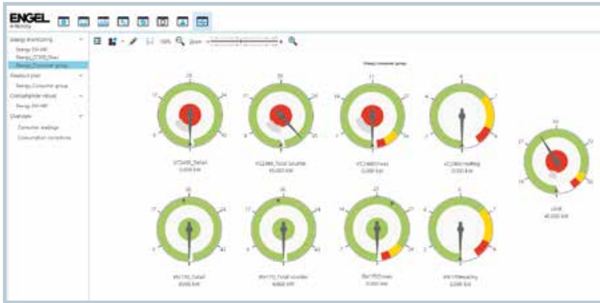
Fig. 5. Machine networking also benefits energy management. The new “energy” module of the MES solution e-factory renders the instantaneous energy needs of individual consumers transparent (© Engel)
