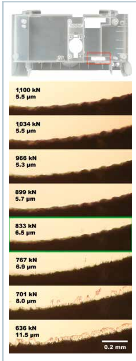
Fig. 3. Burr formation on a medical housing part was investigated in the region of the marked opening. The fine burr that occurs upon clamping force reduction only becomes visible in a transmitted light photograph under a microscope (series of images at the bottom stating the clamping force and peak breathing values). The clamping force as optimized by “iQ clamp control” is 830 kN
