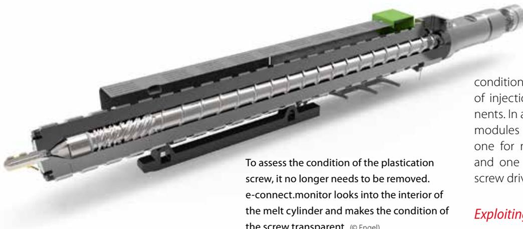
To assess the condition of the plastication screw, it no longer needs to be removed. e-connect.monitor looks into the interior of the melt cylinder and makes the condition of the screw transparent (© Engel)
