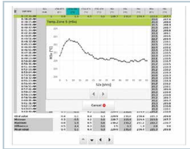
Fig. 4. A quick graph can be generated from the process data log at any time (© Engel)
