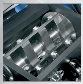
Rotary discs integral with the rotor and containment rings avoid overheating and dust production
