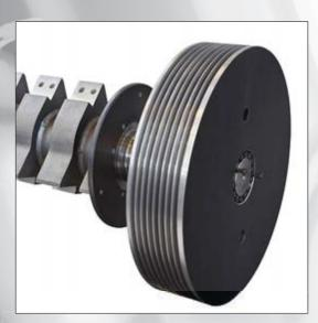
Transmission design gives higher inertia: only 10% of installed power consumed during non productive operation; 30-50% during grinding time
