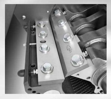
Bench blade setting jig maintains correct gap between fix and rotary blades
