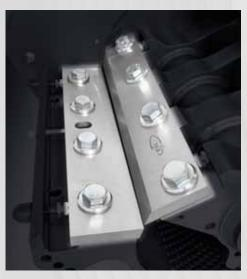
Arrow angle and cutting edge, blades setting to reduce cutting stress
