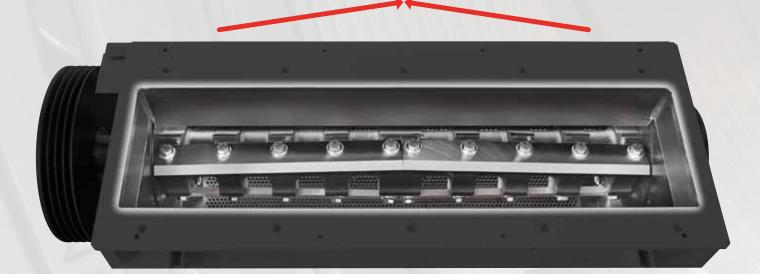
Double roller rotor bearings installed by torque wrench to ensure free and perfect rotor revolution
