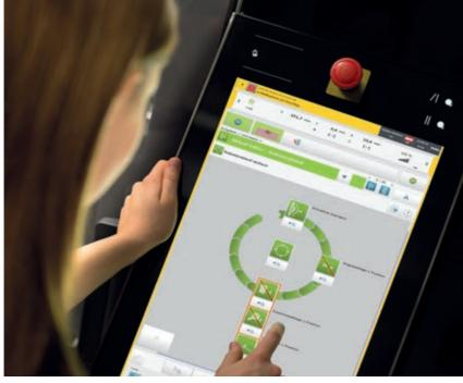
Robot control = machine control: because ENGEL supplies injection moulding machines and robots from a single source, full integration of the two control landscapes is guaranteed without the need for a Euromap 67 interface. The RC 300 robot control unit is integrated into the machine control unit CC 300 as a subsystem.
